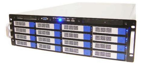
The SB-1 high speed network storage box is capable of sustaining a combined write bandwidth of over 48Gb/s thru the 16 external 10Gb Ethernet interfaces to 32 SATA-2 solid state drives.
